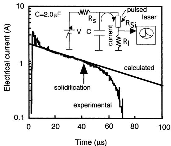
Fig. 1. Changes in the electrical current flowing in 60-nm-thick silicon stripes. The samples were heated by laser irradiation at  $400 \text{ mJ cm}^{-2}$  during application of a voltage at 130 V. Equivalent circuit is shown in the inset. Series resistance  $R_s$ , and load resistance  $R_l$ , were  $1 \text{ k}\Omega$  and  $5 \Omega$ .
