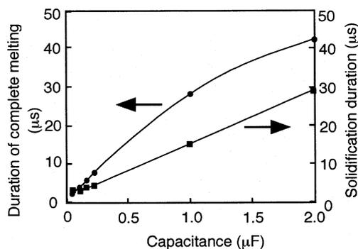
Fig. 2. Duration of complete melting and solidification as functions of capacitance.
