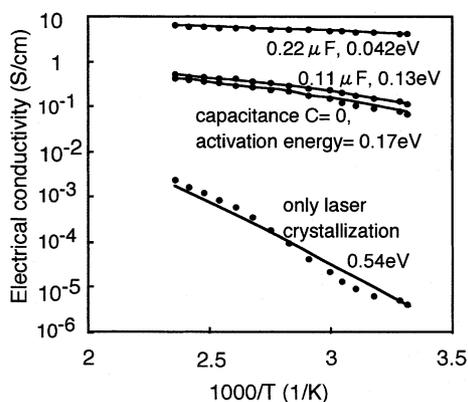
Fig. 4. Electrical conductivity measured (dotted curves) and calculated (solid curves) as a function of reciprocal absolute temperature for  $7.4 \times 10^{17} \text{ cm}^{-3}$  phosphorus-doped silicon films crystallized at 0.11, 0.22  $\mu\text{F}$  and zero capacitance as well as for simple laser crystallization at  $400 \text{ mJ cm}^{-2}$ . Inset presents image of Al electrodes with a narrow gap of 4  $\mu\text{m}$  formed at the edge region of silicon strips after crystallization.
