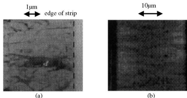
Fig. 3. Photographs of the bright field image at the edge region of silicon stripes crystallized by the electrical current-induced joule heating method with a capacitance of  $0.22 \mu\text{F}$  (a) and of Secco etched films crystallized at  $1.0 \mu\text{F}$  (b).
